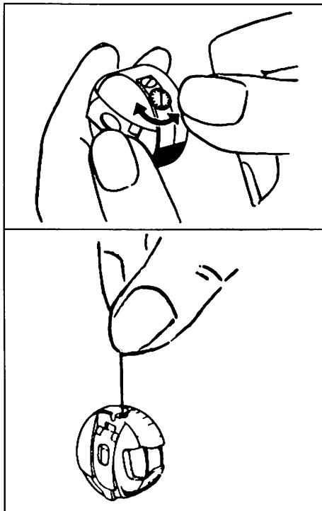
To regulate the bobbin thread tension turn the knurled screw with the tip of your thumb. Turn it counter-clockwise for a weaker tension, or clockwise for a tighter tension.
